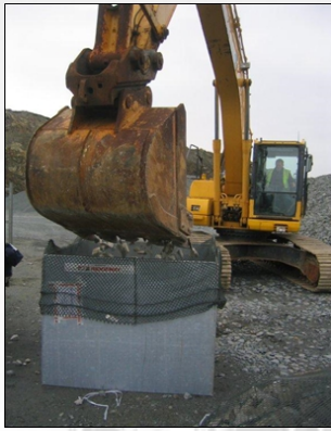
Set filter unit in production frame and fill with stones
